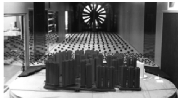
Figure 4: A wind tunnel test of a high density estate in Hong Kong by Consultant RWDI of Canada.
