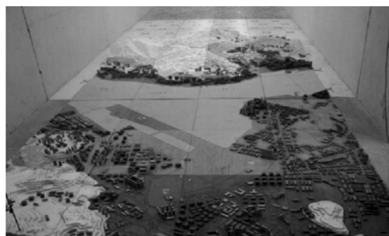
Figure 12: The Old Kai Tak site undergoing wind tunnel site wind availability tests.
